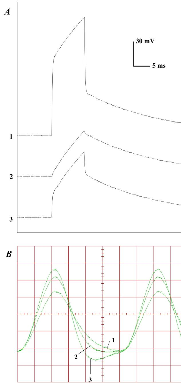
**Figure 4.** How to set the capacitance neutralization during DCC mode
