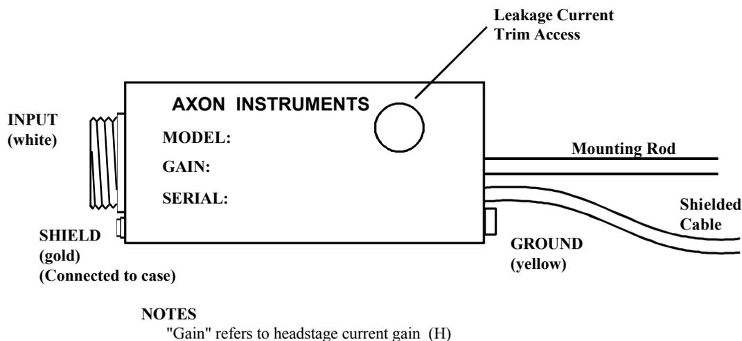
**Figure 14.** HS-2 and HS-4 headstage connection diagram
