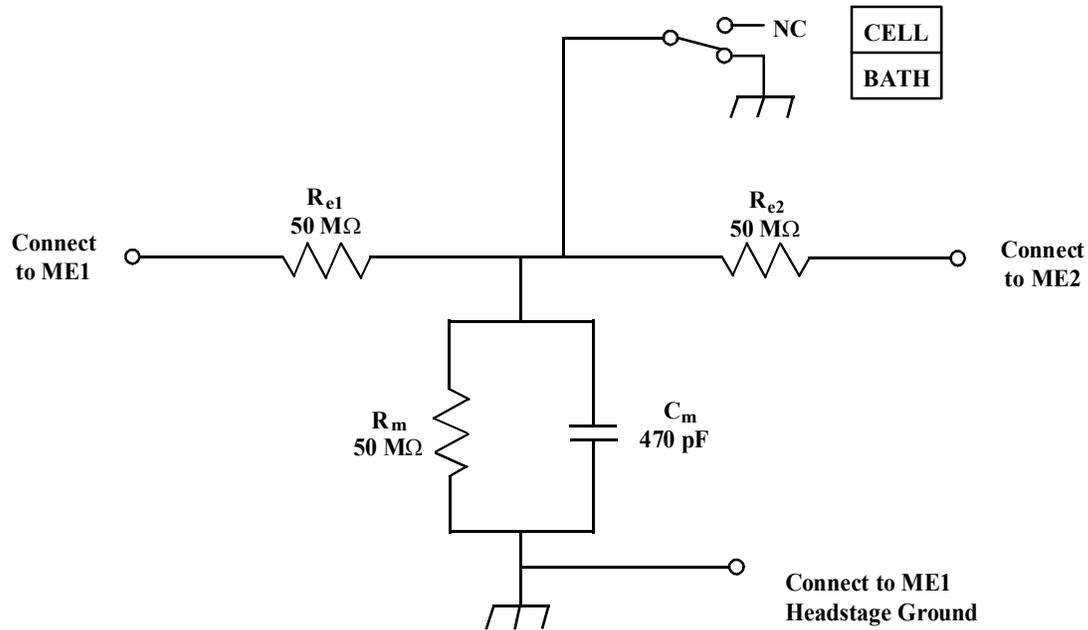
**Figure 10.** CLAMP-1U model cell
