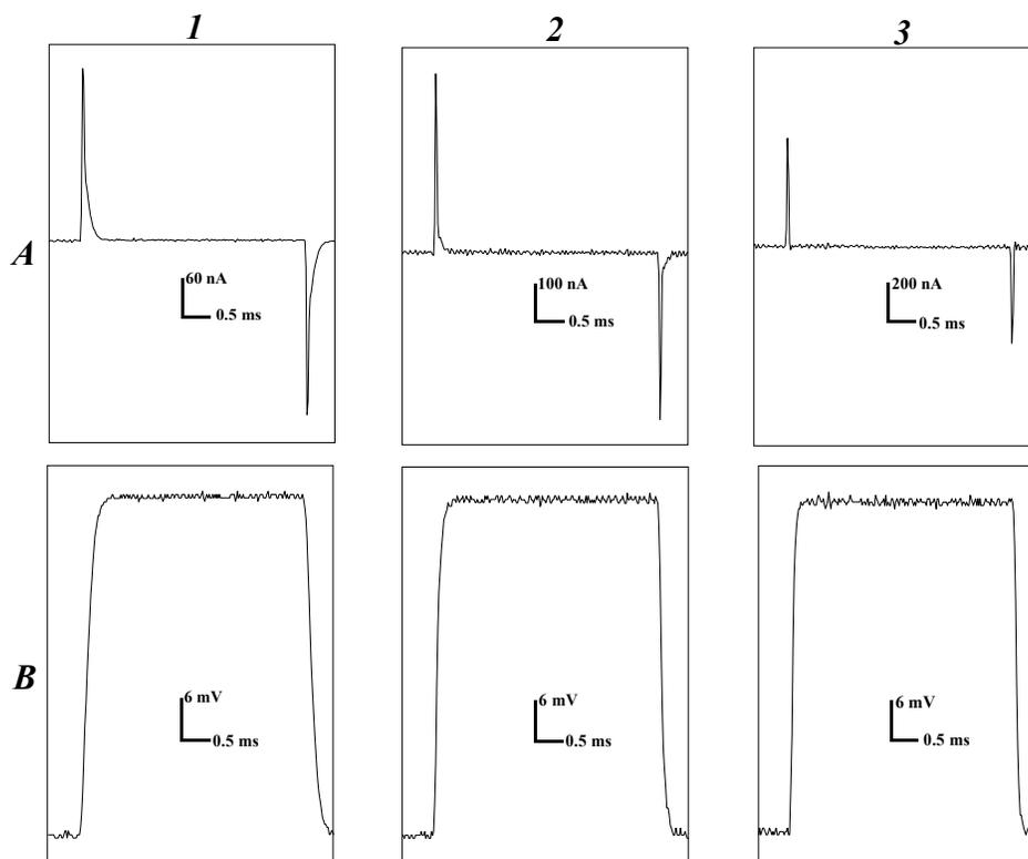
**Figure 7.** Tuning the TEVC with the CLAMP-1U model cell
