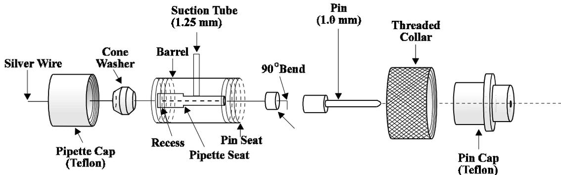
Figure 15. Exploded view of the holder
