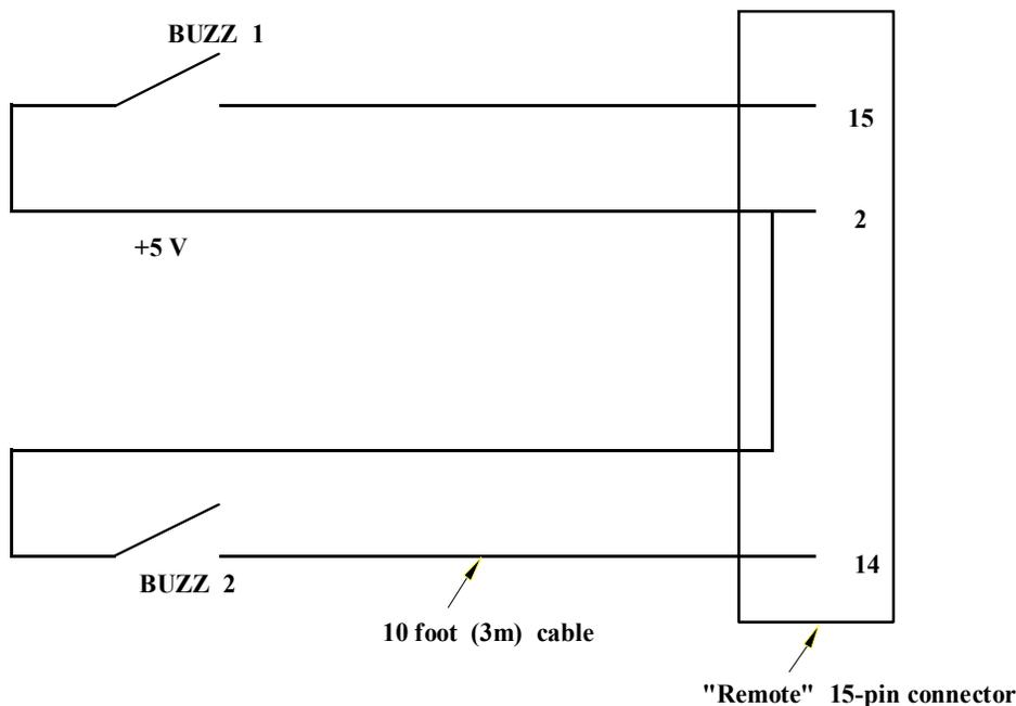
**Figure 18.** External switch wiring diagram
