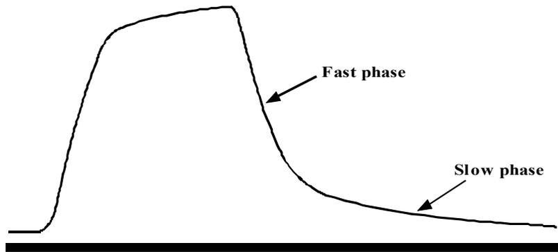
**Figure 9.** Two-phase microelectrode decay
