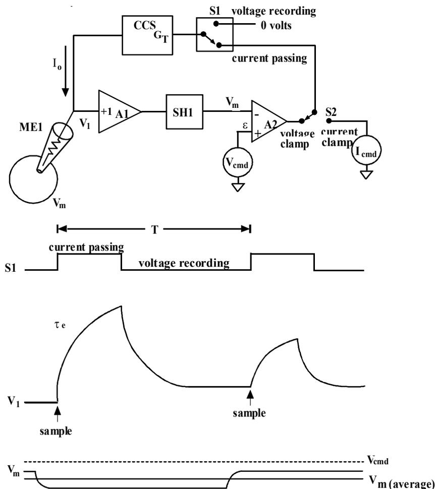
Figure 23. dSEVC block diagram and timing waveforms
