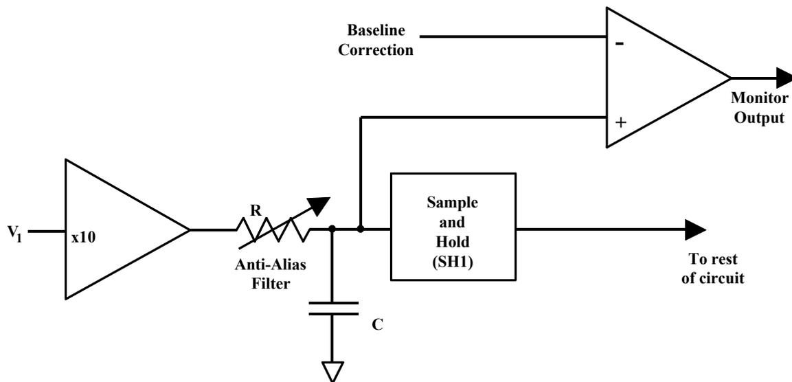
Figure 17. Anti-alias filter and monitor circuit
