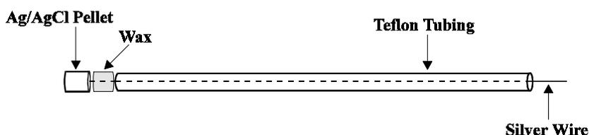
**Figure 16.** Ag/AgCl pellet assembly
